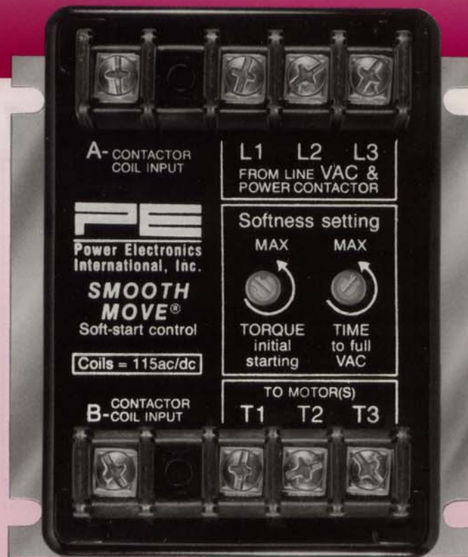
Pictured - SM5A1S - 208 thru 480 vac - 5FLA - smooth control for one or multiple a.c. 3-phase motors up to the rated FLA. 4" x 3-3/4" x 3-3/8" less than 1 lb. UNIVERSAL VAC INPUT allows for easy stocking and wiring!
